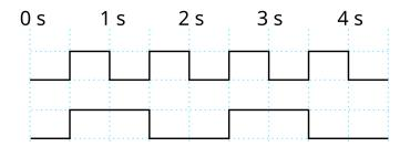
The output frequency is half the input frequency.
