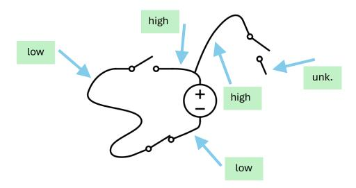
d) What is the voltage at each of the indicated locations in the circuit if every switch is in its active position?
