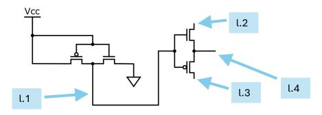
m) What is the voltage at each of the indicated locations in the circuit?
