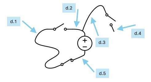
e) What is the voltage at each of the indicated locations in the circuit?
