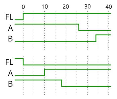
c) In the "Features and benefits" section of the datasheet is the phrase "'break before make' built-in". Don't worry about the specifics, but assume that there are several of the logic circuits above, and the outputs of each circuit (both A and B working together) control electronic switches (one switch controlled by each of these circuits). In this context, "make" means to close a switch and "break" means to open a switch.
