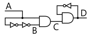
Complete the timing simulation below for nodes B, C, and D in the circuit above using the timing parameters  $T_{PNOT}$ =3 ns and  $T_{PAND}$ =5 ns. Include annotations for the time of each transition, as is done on signal A. There is room at the bottom for additional nodes if desired.
