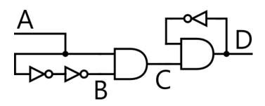
Complete the timing simulation below for nodes B, C, and D in the circuit above using the timing parameters  $T_{PNOT}$ =3 ns and  $T_{PAND}$ =5 ns. Include annotations for the time of each transition, as is done on signal A. There is room at the bottom for additional nodes if desired.
