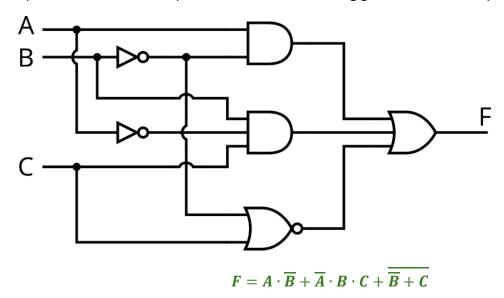
b) Starting with the expression above, draw a starting point for mixed-logic schematic manipulation, then perform a manipulation to create an implementation that uses only NAND gates and inverters.
