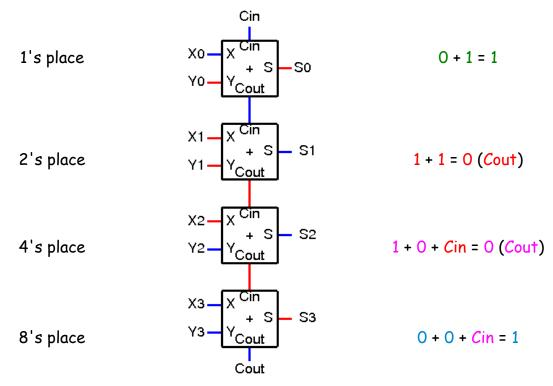
In this example X = 0110 (6) and Y = 0011 (3), Each one bit adder handles one bit position. The collection performs the word addition yielding the correct solution 1001 (9) ... correct assuming an unsigned integer representation. But what about for other representations?
