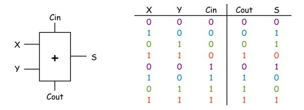
The first case (X = 0, Y = 0, Cin = 1) produces a sum of one. No carry out required. When (X = 1, Y = 0, Cin = 1), the sum is 10 (2). This results in Sum = 0 and Cout = 1. The same outputs occur when (X = 1, Y = 0, Cin = 1). But when (X = 1, Y = 1, Cin = 1), the sum is 11 (3). Carry out moves 10 (2) to the next bit position. The remaining one becomes the Sum output. So the results are Sum = 1 and Cout = 1.
