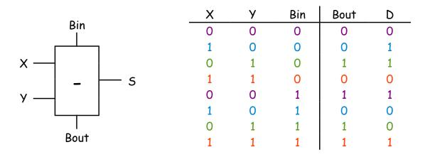
It is interesting to note that difference (D) is exactly the same as sum (S) in addition: odd parity. This makes sense when one considers that, from a single bit position's standpoint, adding one has the same effect as subtracting one. The result toggles. The borrow out expression differs from carry out.
