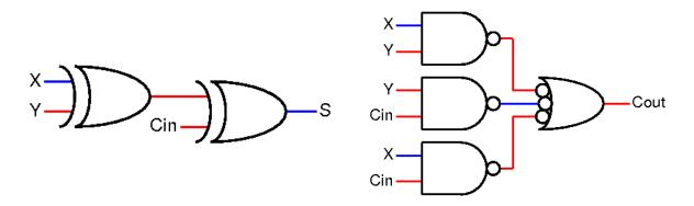
**Going Multi-Bit**: Since each bit position follows the same operations, a multi-bit adder is created by connecting several replicated one bit adders. The carry in of the least significant bit is set to zero. If it is one, an extra one is added to the sum. *This may come in handy later*. Each bit position is implicit relative to its position. Here's a four bit adder:
