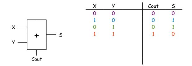
This output is drawn on the bottom rather than the left side of the adder icon because it is used as an input for another one-bit adder. Since the next bit position must process this carry out signal, the adder also needs another input.
