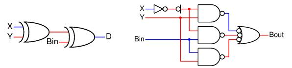
**Two for One**: Full subtracters can be replicated to form a multiple bit subtractor. But that's not how it's done. The hardware cost for subtraction would match the cost of addition. What if there were a way to get both operations using only one multi-bit arithmetic unit? How can an adder subtract? The answer comes from a little math and the magic of two's complement.
