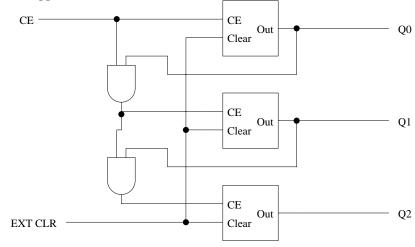
Part C Now use your toggle cells (in icon form) to build a divide by seven counter. This design should include a count enable CE and an active high clear CLR. Your design should clear if (A) the external clear CLR is high, or (B) the maximum output count is reached and the count enable is high. You do not need to draw in the clock signals.
