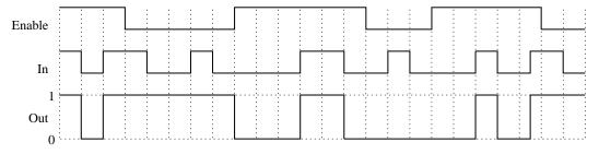
**Part D** Design a latch using two 2-input OR gate, two 2-input NAND gates and two inverters. Be sure to label the signals In, Out, and Enable.
