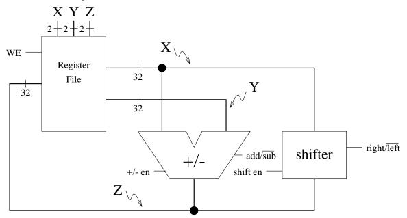
**Part A** Write microcode for this datapath to compute the average of the four initial values in the register file, leaving the result in register zero. You may modify other any register once its value has been summed. Put your answers in decimal (i.e., to select register two on the X bus, put a 2 in the X column).
