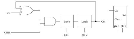
**Part E** Now modify the toggle cell design so that the Clear is active high (i.e., it clears when the input is a '1'), and it only clears when the count enable signal (CE) is high. The truth table below summarizes this behavior. Use mixed logic design methodology. Draw the implementation of a divide by two counter.
