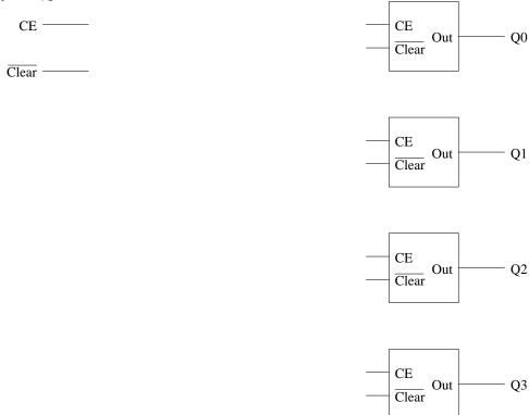
Part C To create a divide by ten counter, logic must be created to detect the 1001 output case and bring low the *Clear* signal. Use a Karnaugh map to determine the simplified expression for the following truth table. Circle all prime implicants.
