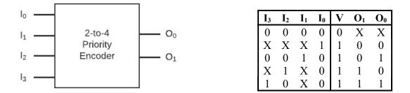
What input priority has been assigned to the four inputs (I<sub>3</sub>, I<sub>2</sub>, I<sub>1</sub>, and I<sub>0</sub>)?
