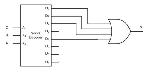
PART B (10 points) How many transistors would you need to implement the circuit above? Assume that the decoder is implemented using canonical sum-of-products equations (no minimization), complemented inputs are provided inside the decoder, and logic gates have no limit on the number of gate inputs.
