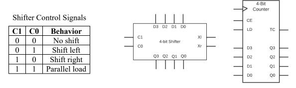
PART A (10 points) Design an 8-bit rotate register (without carry) using the 4-bit bidirectional shifters above.
