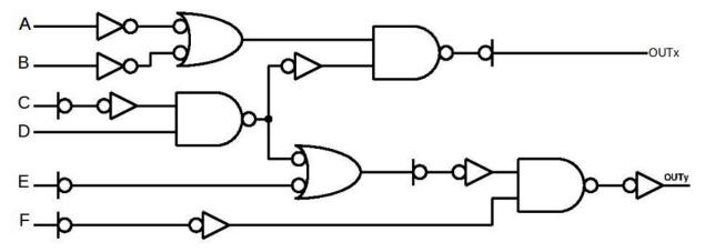
Part A (10 points) Write the output expression for the gate design shown above. Also determine the number of transistors used in its implementation.
