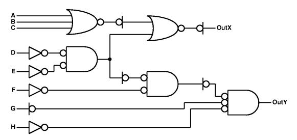
Part A (10 points) Write the output expression for the gate design shown above. Also determine the number of switches used in its implementation.
