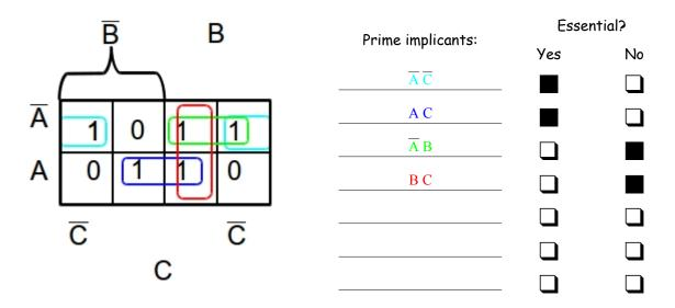
simplified *SOP* expression  $\overline{A \cdot \overline{C} + A \cdot C + \overline{A} \cdot B}$  or  $\overline{A \cdot \overline{C} + A \cdot C + B \cdot C}$ Part B (10 points) Simplify the following SOP expression using a Karnaugh Map. Circle and list all the prime implicants, indicating which are essential and write the *product-of-sums* (POS) expression.
