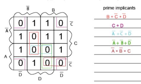
simplified POS expression  $(C+D)\cdot(B+\overline{C}+\overline{D})\cdot(\overline{A}+\overline{B}+\overline{D})$
