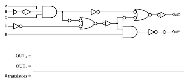
Part B (14 points) Now reimplement these expressions using NAND gates and inverters. Use proper mixed logic notation. Determine the cost of this implementation (in transistors).
