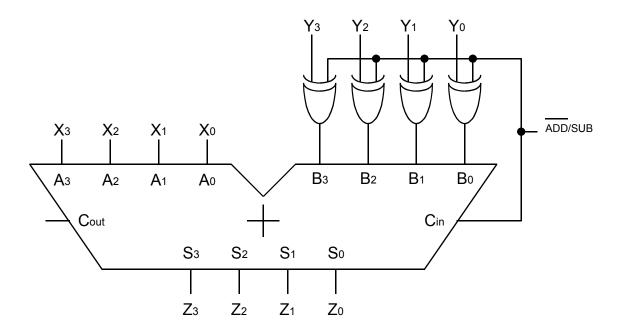
Part C (6 points) Write two Boolean expressions indicating signed two's complement addition and subtraction overflow using inputs  $X_3$ ,  $Y_3$ ,  $Z_3$ . These SOP expressions should be true when overflow occurs.
