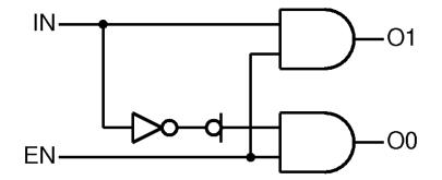
Part C (10 points) Using *only* the three 1 to 2 decoders shown below, implement a 2 to 4 decoder with an enable. Label the decoder inputs ( $IN_1$ ,  $IN_0$ , EN) and outputs (O0, O1, O2, O3).
