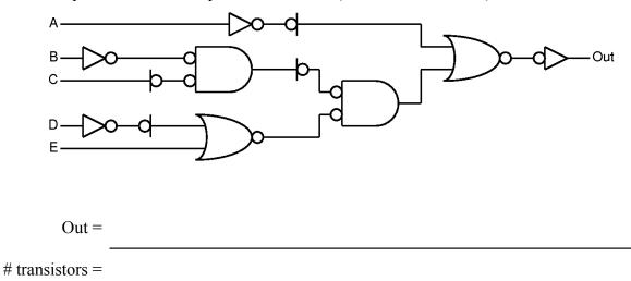
Part B (10 points) Now reimplement this expression using NAND gates and inverters. Use proper mixed logic notation. Determine the cost of this implementation (in transistors).
