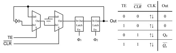
Part B (10 points) Now combine these toggle cells to build a **divide by seven** counter. Your counter should have an external clear, external count enable, and three count outputs O<sub>2</sub>, O<sub>1</sub>, O<sub>0</sub>. Use any basic gates (AND, OR, NAND, NOR, XOR & NOT) you require. Assume clock inputs to the toggle cells are already connected. Your design must support multi-digit systems.
