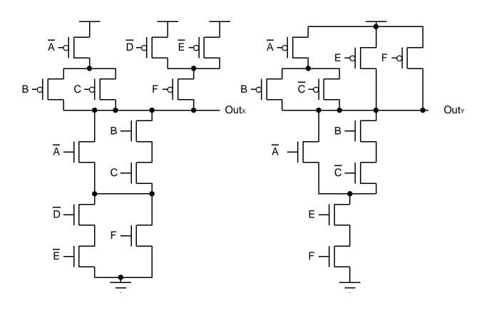
$$OUTx = A \cdot \left(\overline{B} + \overline{C}\right) + \left(D + E\right) \cdot \overline{F}$$
