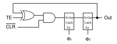
Part B (8 points) Now combine these toggle cells to build a **divide by 24** counter. Your counter should have an external clear, external count enable, and five count outputs  $O_4$ ,  $O_3$ ,  $O_2$ ,  $O_1$ ,  $O_0$ . Use any basic gates (AND, OR, NAND, NOR, & NOT) you require. Assume clock inputs to the toggle cells are already connected. *Your design should support multi-digit systems*.
