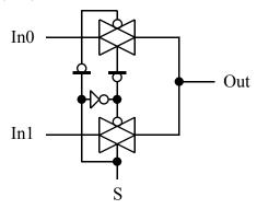
Part C (8 points) Using the 2 to 1 mux implemented in part B (in icon form), implement a 4 to 1 mux. Label all inputs  $(In_0, In_1, In_2, In_3, S_0, S_1)$  and output (Out)
