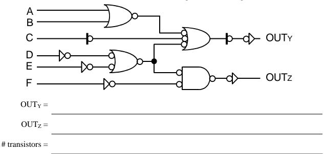
Part B (10 points) Now reimplement this behavior using more efficient multi-input **NOR** gates and inverters. Your design must properly employ mixed logic methodology. Determine the number of switches required for this *improved* implementation.
